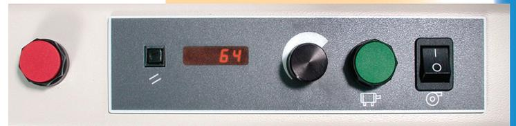
Both units are equipped with interlocks for fault detection and safety, variable speed control and a five-digit resettable counter for job auditing.
